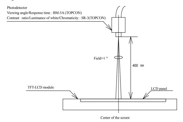
Fig.3 Optical characteristics measurement method
